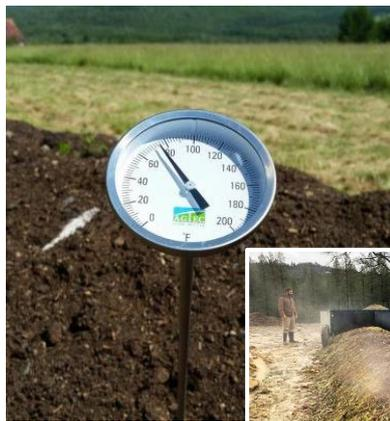
1. A temperature thermometer / probe capable of reading compost temperature between 40 and 100 °C. Temperature readings should be taken from the centre of the pile.
